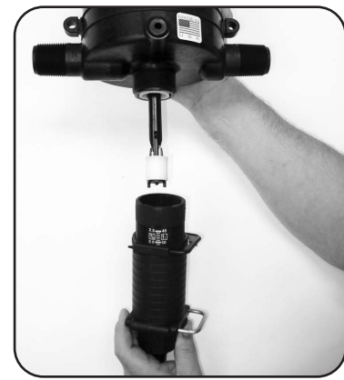
Step 8. Screw LOWER END CYLINDER ASSEMBLY onto body. Ensure #16 gasket is seated on the top of cylinder assembly.
