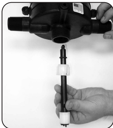
Step 6. Reinsert #15 SEAL RETAINER and #17 O-ring onto # 51 SHAFT ASSEMBLY.
