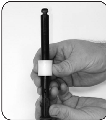
Step 5. For 2.5% & 5% Replace #44 DOSAGE PISTON flared-end up and #14 O-ring. 0.3% only: Replace # 51 SHAFT ASSEMBLY. See Step 5a.
